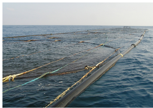
Subflex cages – submersible single-point mooring flexible net cage system
